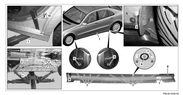
Shown on model 211.0 on left longitudinal member paneling
