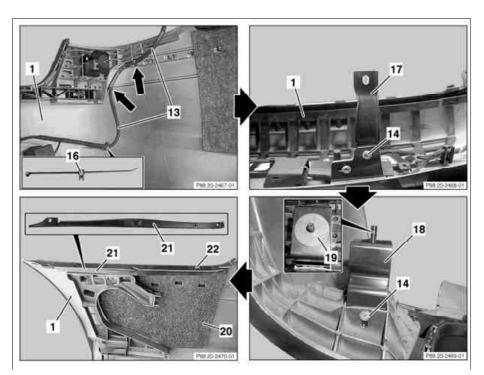
Fasten guide rails (21) to bumper (1) on left and right each with plastic rivet (22)
